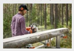
Special longitudinal cut Saw Chain for use on longitudinal cut tools as well as mobile small sawmills. Half-chisel tooth Chain with high cut quality, with a low level of vibration and soft cutting characteristics.
