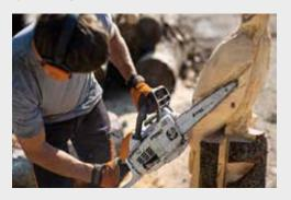
Special Saw Chain for wood carvers. Minimum vibration, very good cutting performance, shortened cutter top plate means it is not necessary to apply pressure when piercing, capable of a noticeably better piercing speed compared to conventional 1/4" Saw Chains.
