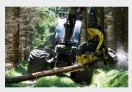
Saw Chain for use on special machines in mechanical wood harvesting and firewood preparation, robust and durable. Reduced tensions result in low levels of crack formation with low wear and a particularly long service life. Must not be used on hand-guided Chainsaws.
